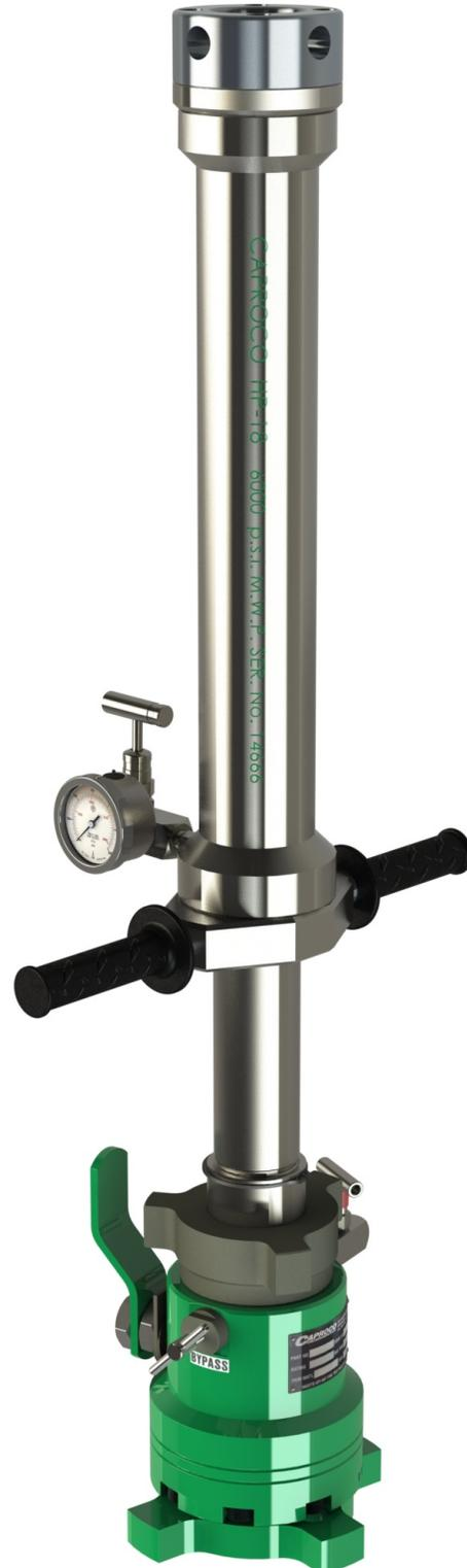
The service valve provides a temporary seal at the access point while the monitoring device is removed for inspection, maintenance or service. A key advantage to the Caproco service valve's design is that it can swivel even once tightened onto the access fitting, so that the operator may orientate it in a position that gives clear access to the bleed-port and drain valves and handle, taking into account any encumbrances that may be present in the working space.
